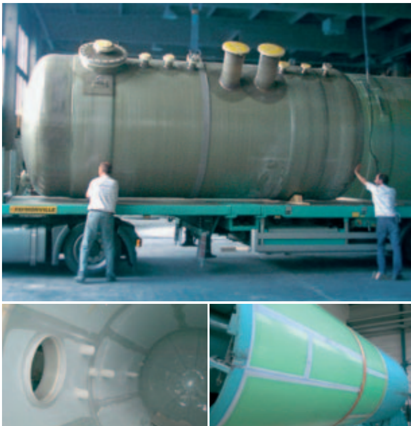
GFRP composite tanks are six metres long and 2.4 metres in diameter. The SIMONA® PVDF-GK sheets are clearly visible in the construction phase (below).
