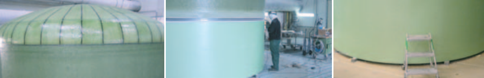
Illustrations from left to right: Tank cover, manufacture of the cylindrical section, tank base
